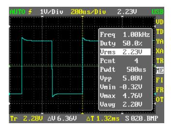
The highlighted/selected measurement (**Vrms**) is duplicated on the top bar for reference when the popup is closed.
