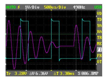
The cyan square wave is a trace of the live input signal and the magenta waveform is a static reference waveform.
