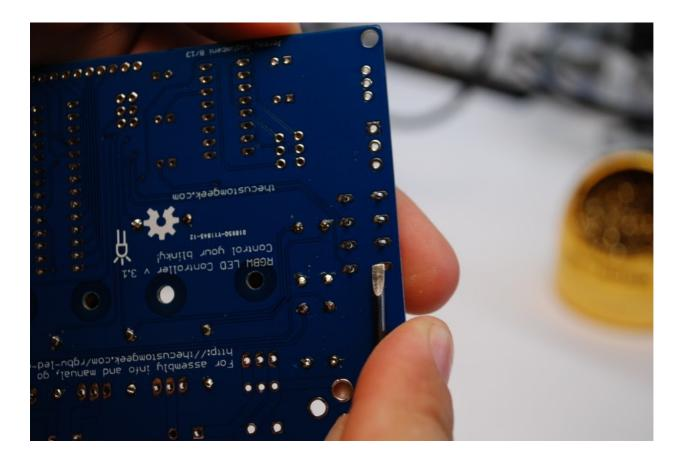
Insert the white LED as shown, the flat side of the LED will be the shorter lead, this is the negative side. It will match the silkscreen on the board.
