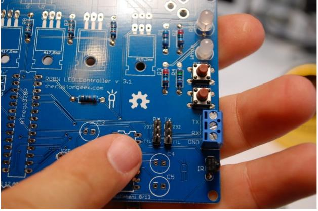
Next, insert and solder the 5 .1  $\mu F$  capacitors to the board as shown. Note the longer lead, the anode, goes in the square hole.
