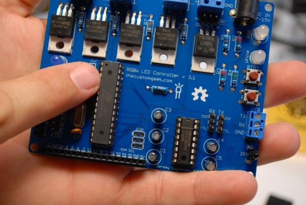
Next, install the jumpers on the voltage and serial select headers.
