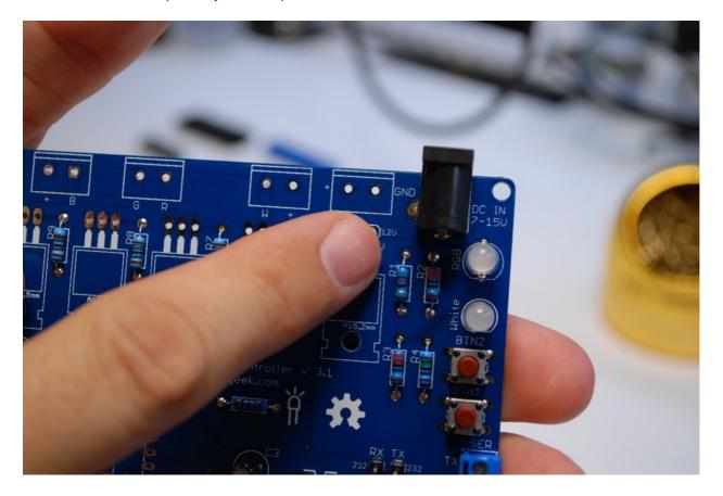
Next, install and solder the 7805 voltage regulator. make sure you use the 7805 and not a IRLB8721PBF MOSFET! They have the same package. ;)
