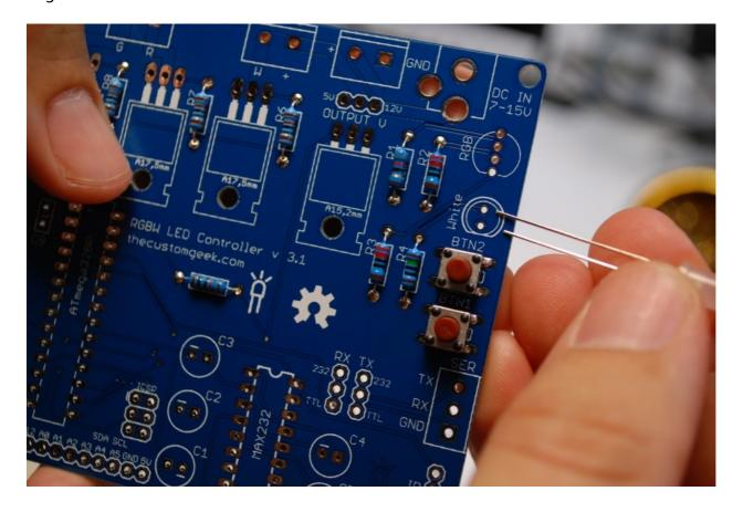
Insert the RGB LED as shown, shortest lead next to to flat side as marked on the silkscreen.
