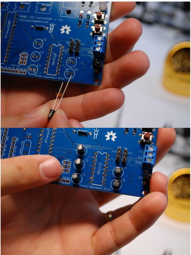
Next, solder the 16 pin DIP socket for the MAX232. Note the notch at the top. We can do the same lead bending trick as we did with the switches. This will help us keep a low profile as well as keep the socket in place while we turn the board over to solder it in place.
