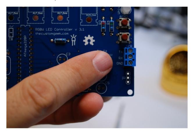
Next, solder the IR sensor as shown, with the rounded side facing out.
