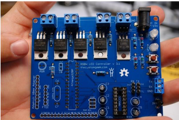
Next, solder the 28 pin DIP socket in for the ATmega328. Note the notch at the top.
