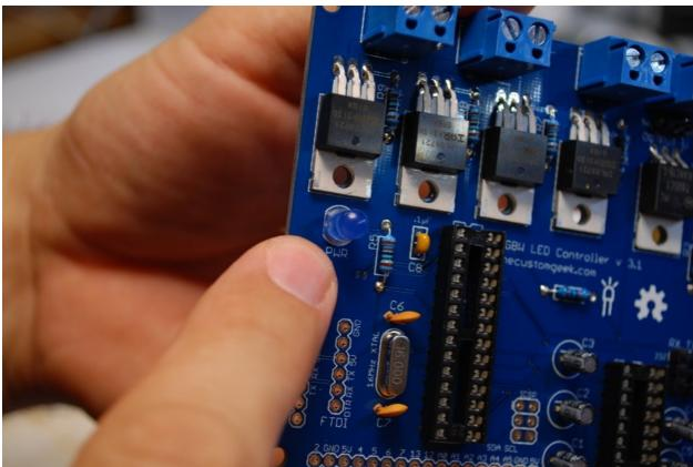
Next, solder a 6 pin male header in the FTDI spot as shown.
