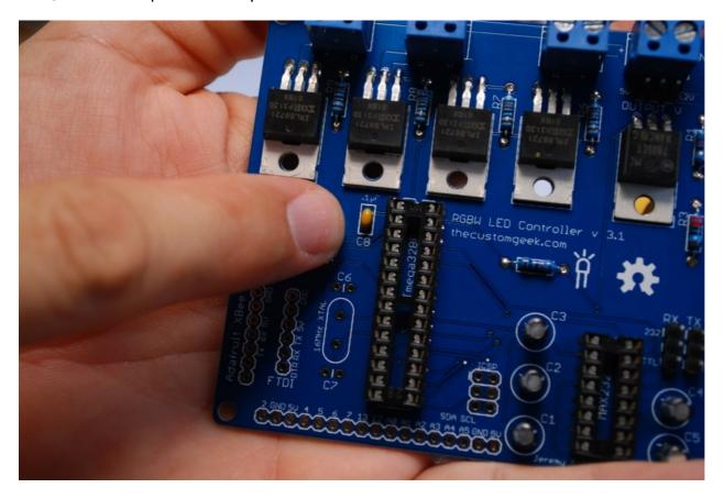
Next, solder the 16MHz crystal. It is not polarized, it can go in either direction.
