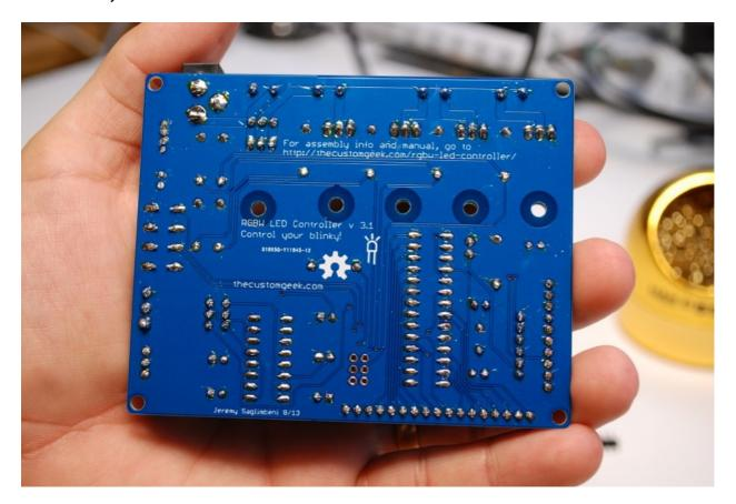
Next, we will insert the ATmega328 and MAX232. You will need to bent the row of pins in slightly for them to fit into the DIP sockets. Make slight adjustments and check the pin spacing often.
