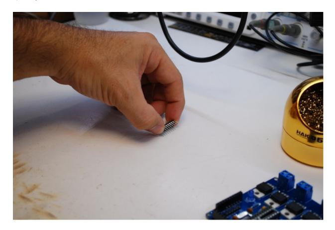
Make sure the notch on the MAX232 IC is toward the top as shown below.
