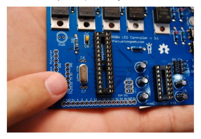
Next, solder the two 22pF ceramic capacitors on both sides of the crystal.
